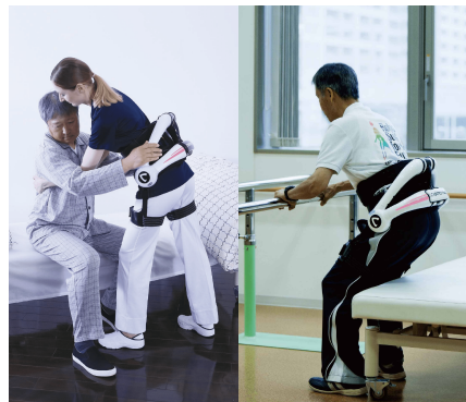
New version of HAL that could be used for dual purpose: to support both care givers and care receivers
