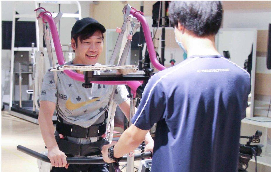
Neuro HALFIT session at Tsukuba Robocare Center (using HAL Lower Limb Type for gait training)
