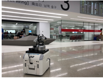
Spraying antiseptic solution in terminal building
