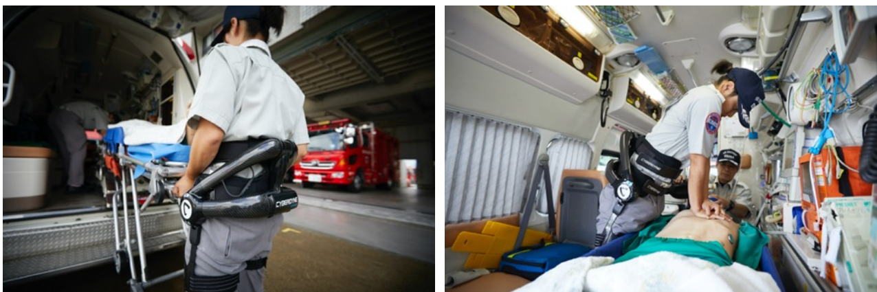
Paramedic training their task while wearing HAL Lumbar Type for Labor Support (credit: Ebina City Firefighting Department)
